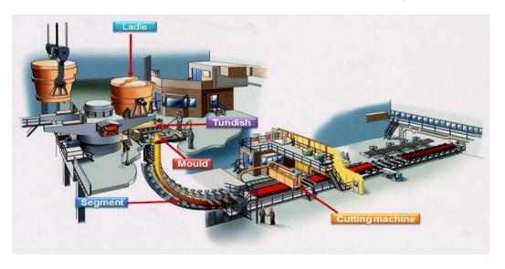
Potential hazards identified during caster operation are free flow of liquid metal from holding vessels like ladle, tundish. Mould Breakouts leading to metal spillage in caster machine causing fire hazard. Hot surface exposure are prone to burn injury caused during this operation
